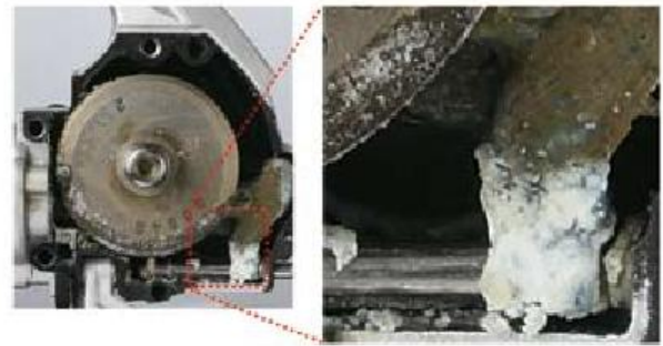
Comparison of reels with/without MAG SEALED. Source: DAIWA Intern. Service Dept.
