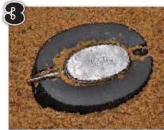
Carefully position the Method Feeder in centre of the mould and press firmly.
